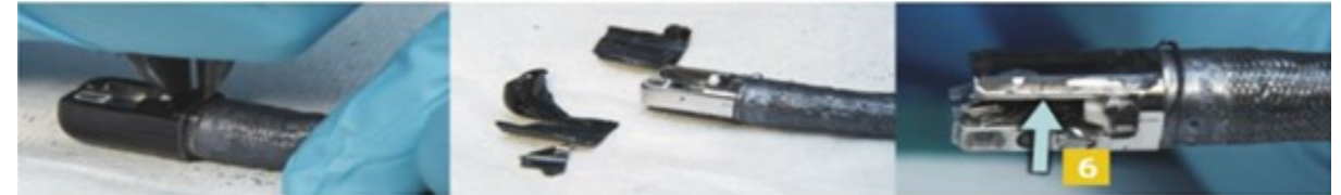
c. trimming the tip cover
