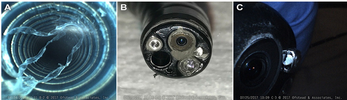
Fig 4. Visible defects observed during visual inspections. (A) Non-intact channel lining in gastroscope B-2; (B) damaged distal end with exposed metal mesh fibers protruding from gastroscope C-1; and (C) white debris protruding from the water jet outlet on the distal end of gastroscope C-3.
