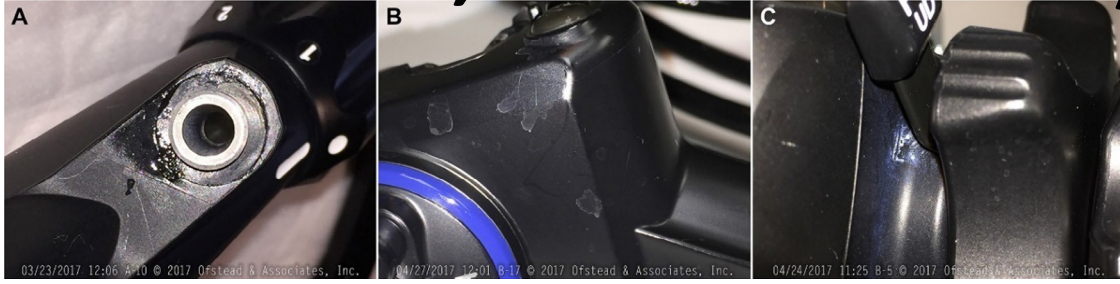
Fig 2. Residues observed on external surfaces of endoscopes. (A) Oily residue near biopsy port of pediatric colonoscope A-10; (B) dried “water spots” on control handle of cystoscope B-17; and (C) whitish-blue, powdery residue under control handle knobs of gastroscope B-5.
